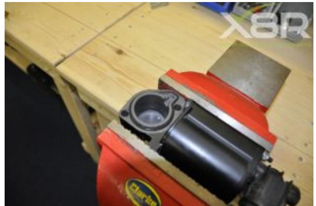
Remove old seal from inside of head, clean groove and mating surfaces and replace with the correct seal from our kit, please note some compressors use an O-ring seal others use a shaped seal, we include both in our set, you only need to use one of these. Check cylinder for any damage; the cylinder is tapered, check for dents or scratches these can significantly reduce the life of replacement piston seals.
