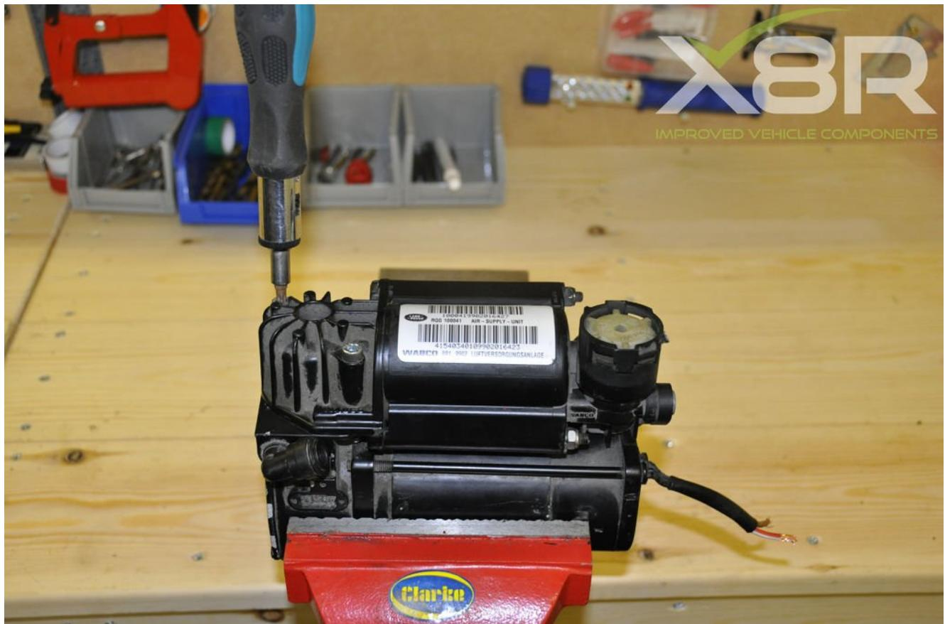
Clean the outside of the compressor to stop any debris entering the internals of the compressor.
