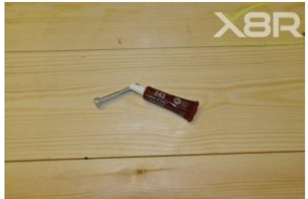
Clean all mating surfaces and refit head. Install our new bolts applying a little lock tight to the threads. Refit temperature sensor if one was fitted.
