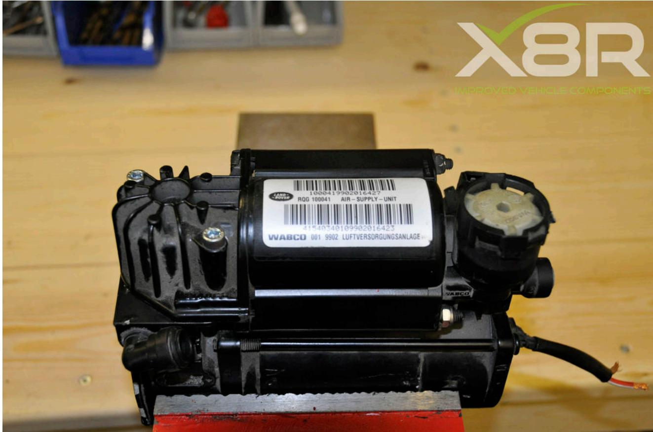
It is very common that the piston ring seal within the Wabco compressor wears down reducing compressor performance leading to noisy, slow rising or even inactive air suspension.
