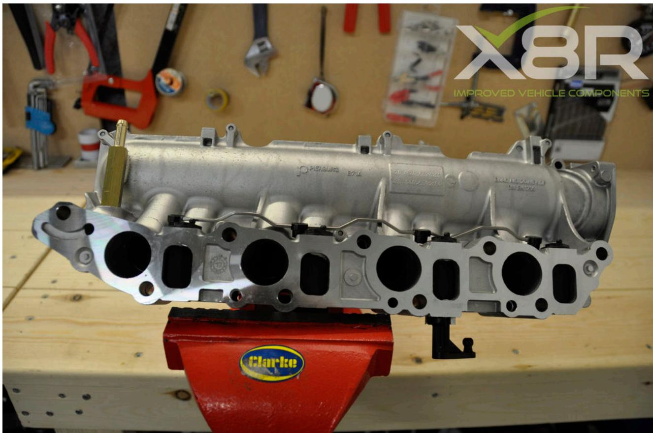
Refit operating rod. Push down on rod to secure using long reach pliers or reshape coat hanger hook to push down on rod.
