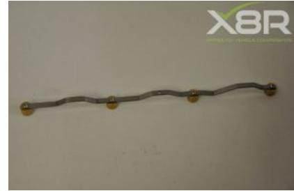
Add thread-lock to the screw threads and attach the bushes to the rod as shown.
