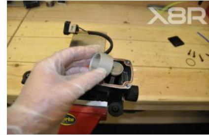
Remove 4 bolts on cylinder head, it is good practice to label each bolt so that they can be refitted in their original position. Use a socket rather than a Torx screwdriver to remove as the bolts are relatively soft.
