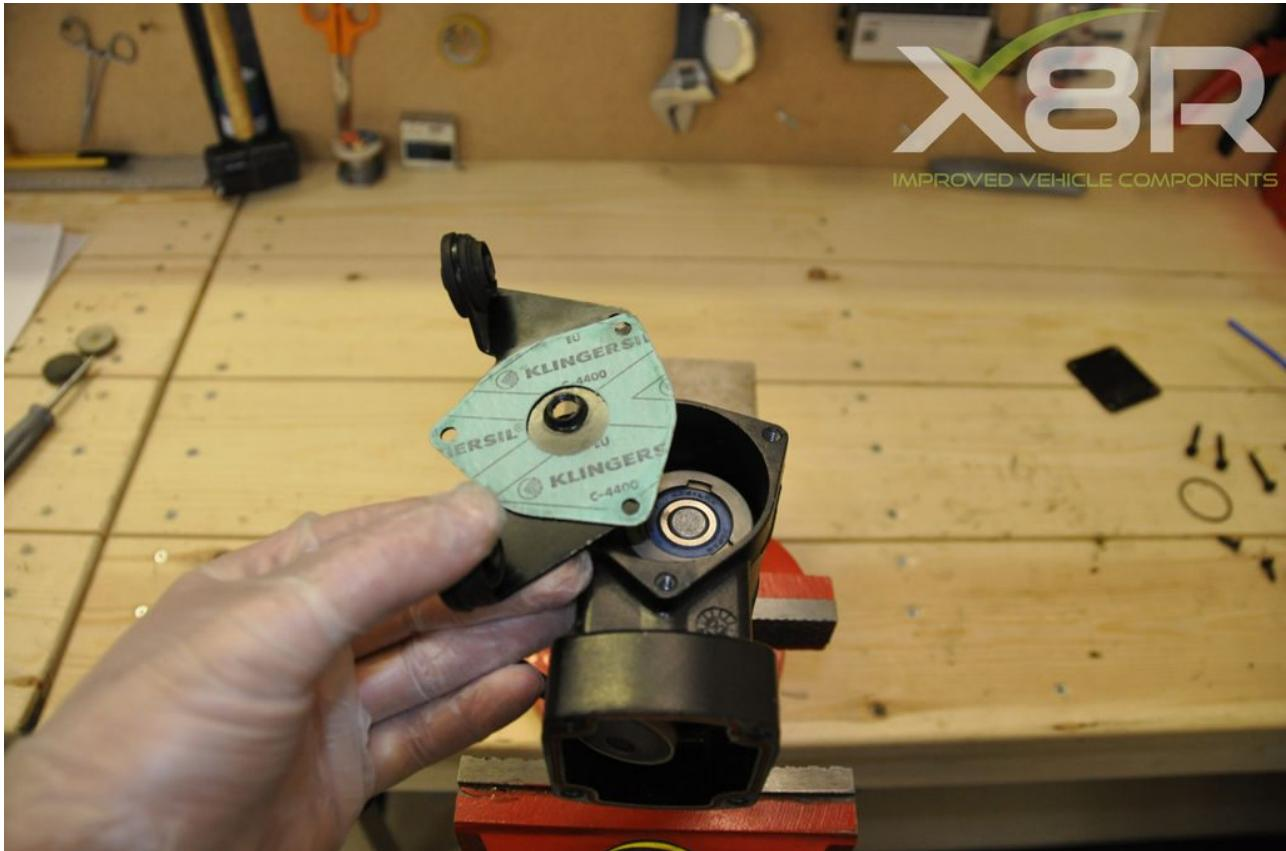
Again using a socket and remembering location for respective bolts remove 3x bolts on face plate.
