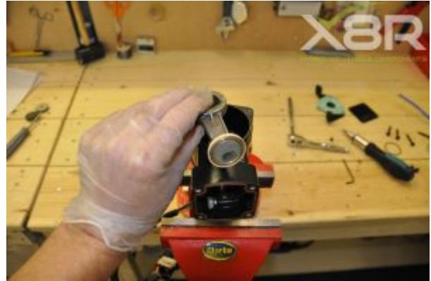
Remove grub screw shown on side of compressor.
