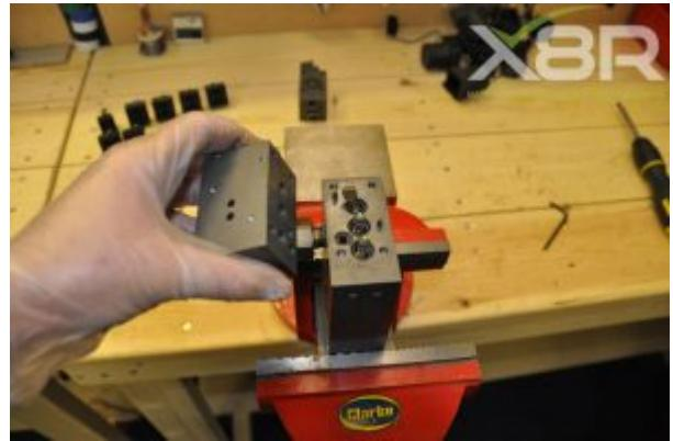
Remove 4x Allen bolts shown and lift off block.
