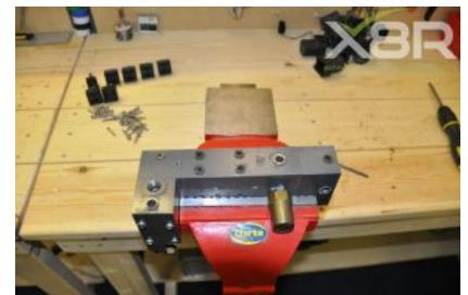
Fit O-rings in to airline holes, each hole takes 2x O-rings, it will be evident which holes take which sized O-rings.
