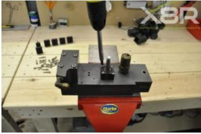
Label solenoid bases 1-7 and remember orientation for re-installation.
