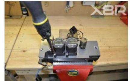
Label solenoid covers 1-7 and remember orientation for reinstallation.
