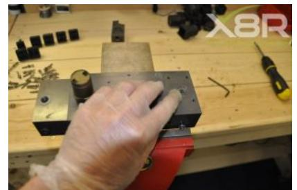
Remove 4x Allen bolts and remove diaphragm block.
