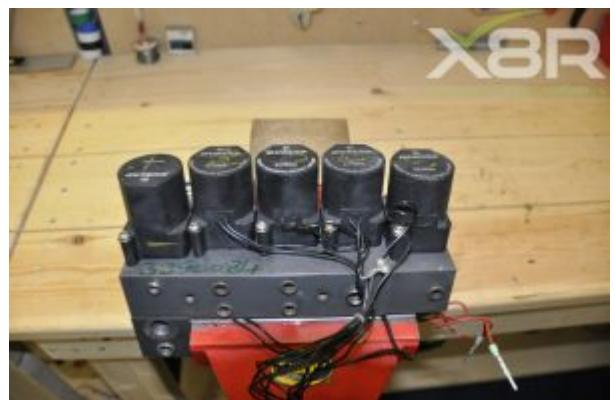
Refit solenoids and covers in same place and orientation as removed, remove any labels attached at start to remember orientation.
