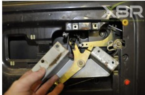
Remove pivot point which prevents door lock mechanism removal.
