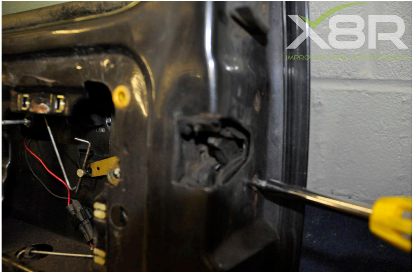
Remove screws retaining lock mechanism.
