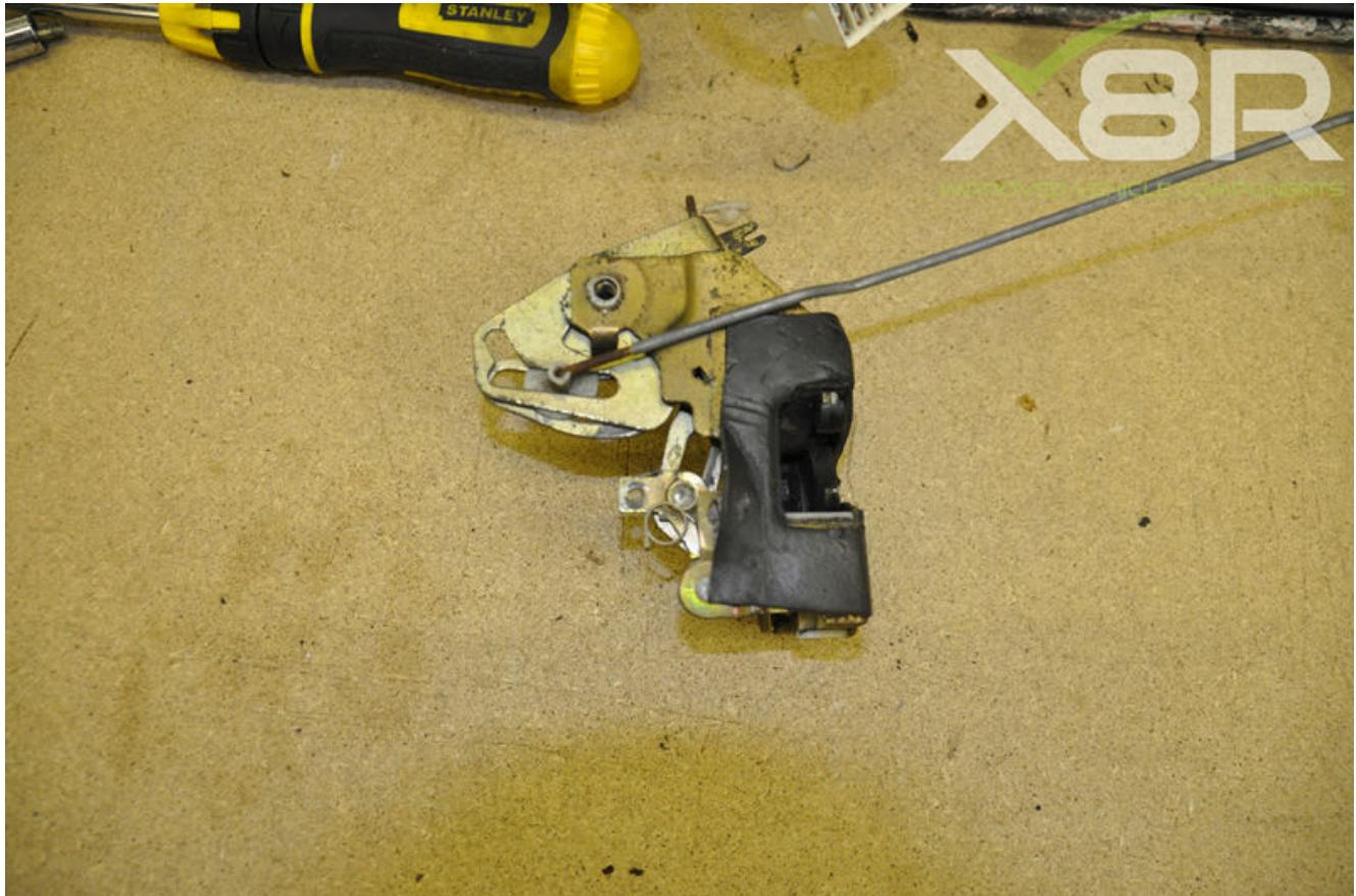
Position lock as shown, you will see from image where spring should be located, remove remains of old spring if evident.
