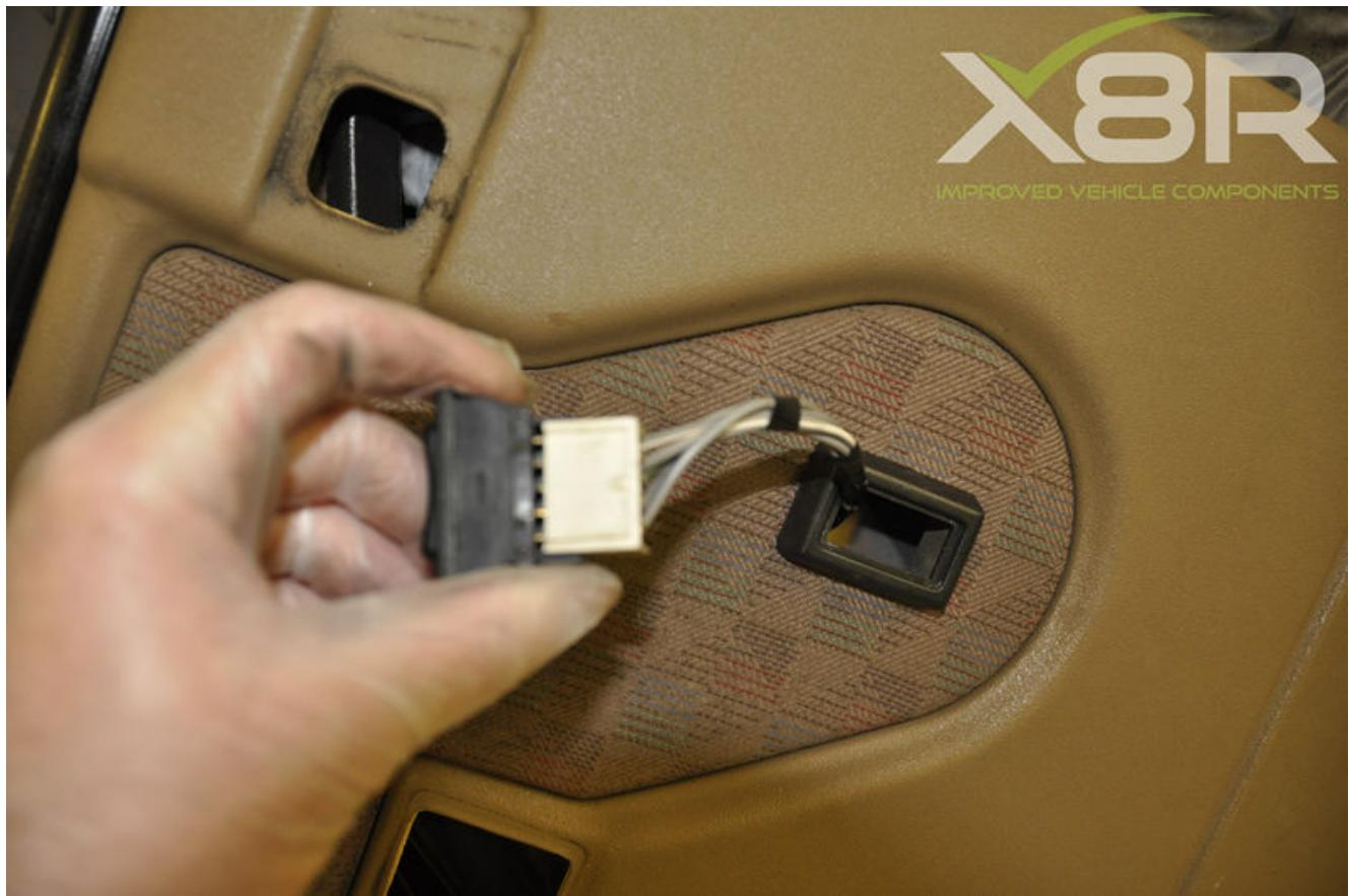
Lift the door trim up over the lock pin and disconnect the window switch.
