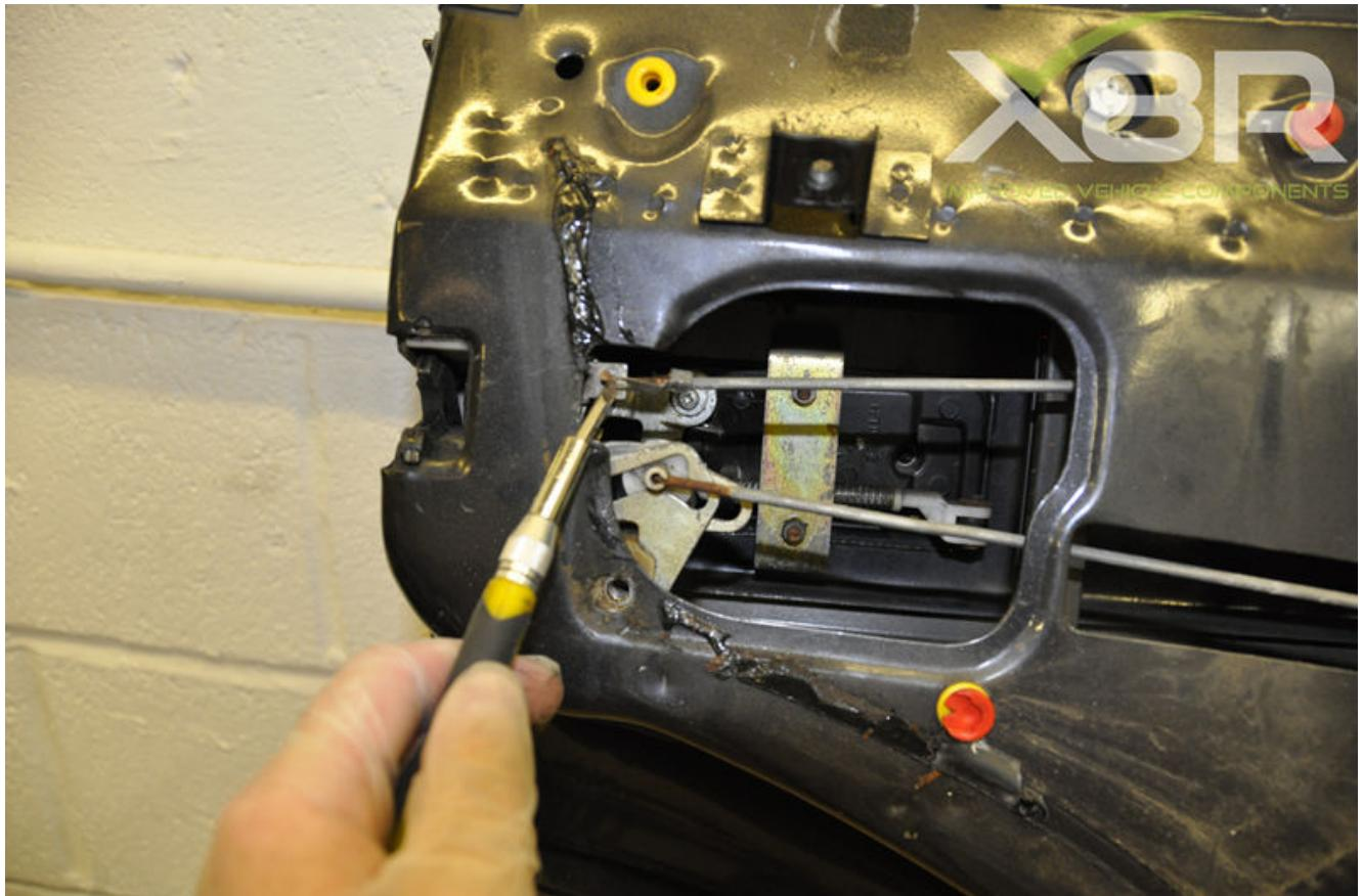
Remove the top front linkage, lift the clip off of the rod, retain this for reinstallation, push the rod away from the locking mechanism.
