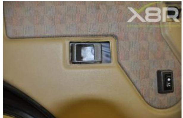
Remove the latch lever plastic surround by holding open the lever and unscrewing the screw underneath. Slide the plastic trim out.
