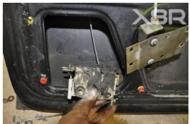
Disconnect toothed clip with small pliers and remove linkage.
