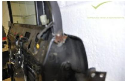
Loosen window frame by removing the two bolts shown.
