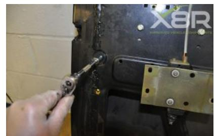
Unscrew the latch lever and twist linkage out of position
