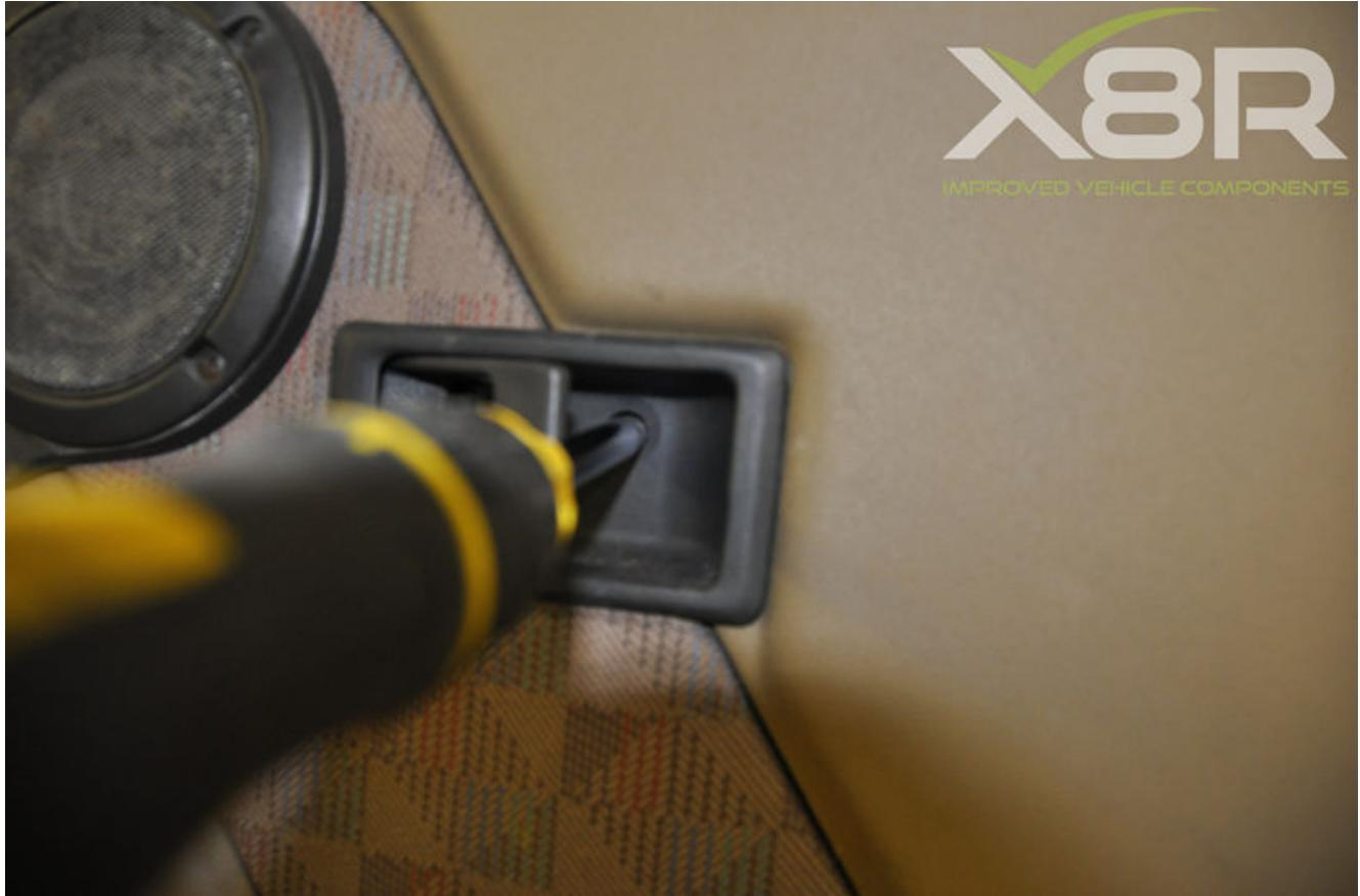
Remove the latch lever plastic surround by holding open the lever and unscrewing the screw underneath. Slide the plastic trim out.
