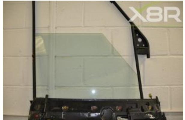
Disconnect electrical connectors to the mirror and carefully lift the window frame
